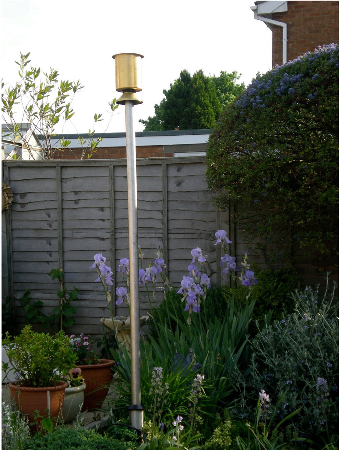
Figure 1: Pole mounted fieldmeter for continuous long term measurements
