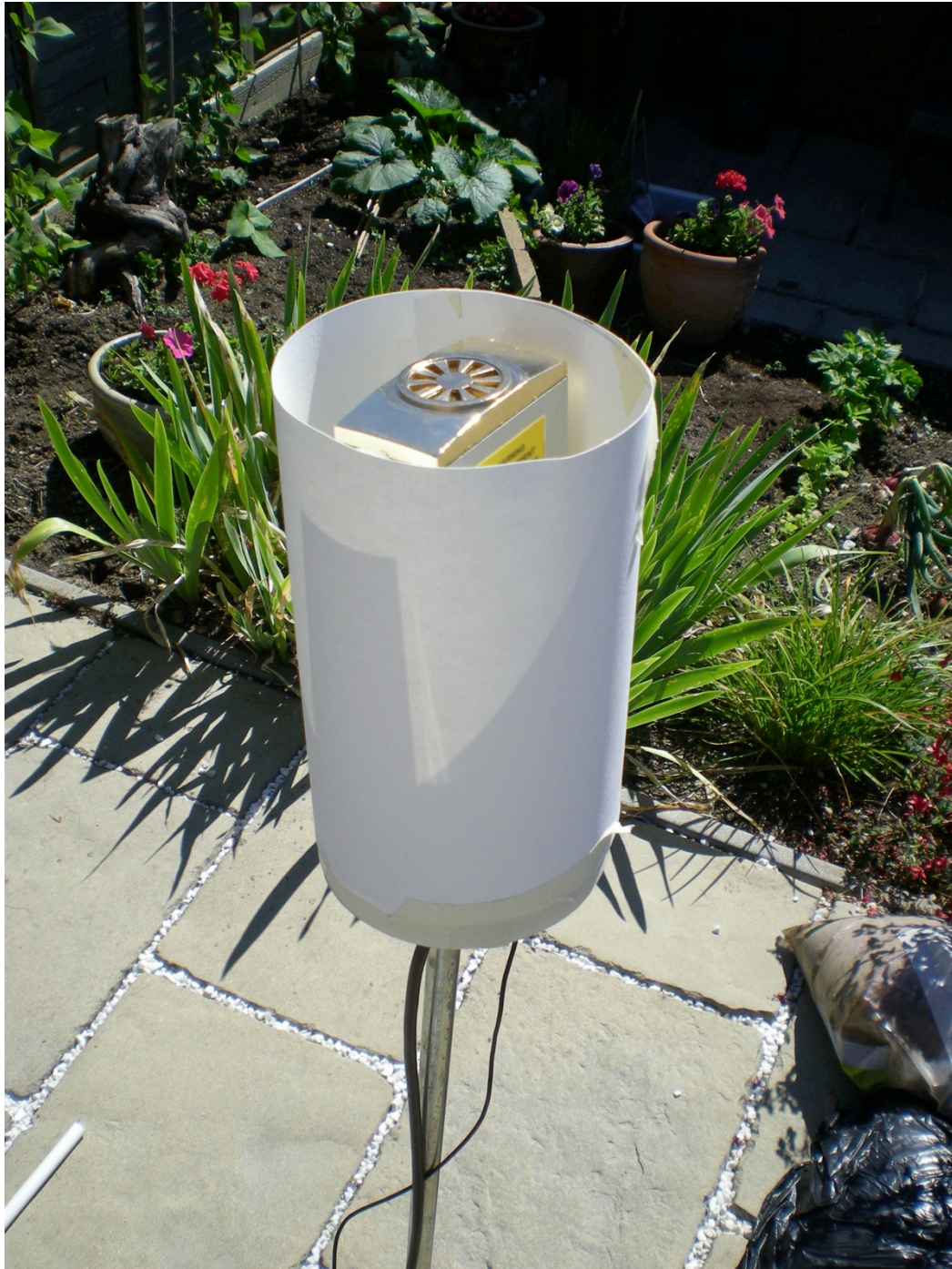
Figure 7: Fieldmeter with shield increasing diameter to about 105mm
