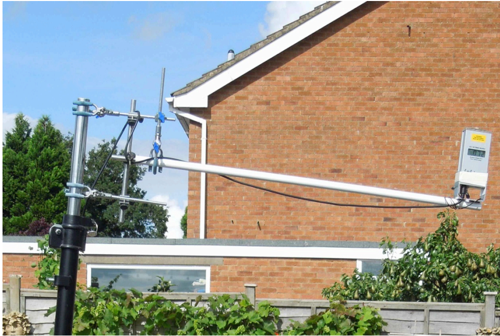
Figure 4: Photograph of the experimental arrangement for examining the influence of the fieldmeter pointing direction and height
